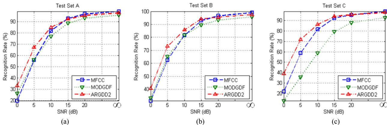
**Fig. 3.** The recognition rates of the ARGDD2-E\*, MODGDF-E\*, and MFCC-E versus SNR on the AURORA 2.0 task (the best cases for each feature based on Table 1). (a) Test set A (includes subway, babble, car, and exhibition additive noises), (b) Test set B (includes restaurant, street, airport, and train-station additive noises), (c) Test set C (includes subway and street convolutional noises).
