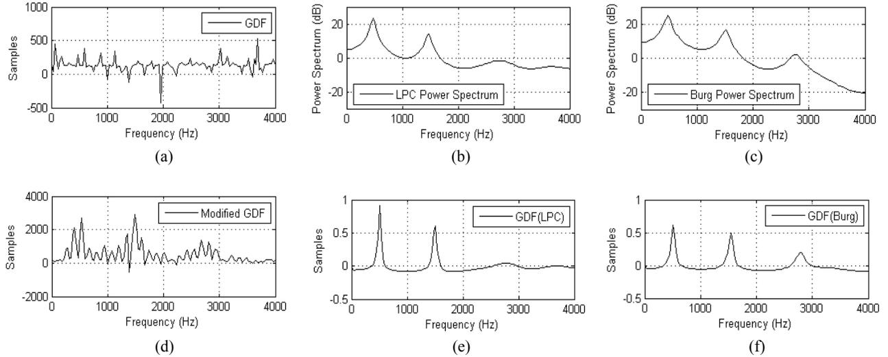
**Fig. 2.** (a) Group delay function, (b) LPC power spectrum, (c) Burg power spectrum, (d) modified group delay function, (e) GDF (LPC), (f) GDF (Burg).
